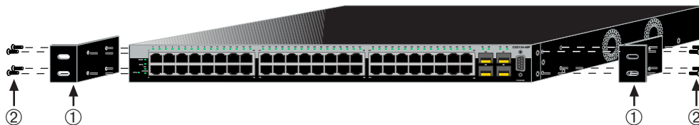
Figure 3-5 Attaching the Rackmount Brackets
